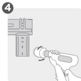
Drill Wall Hole
